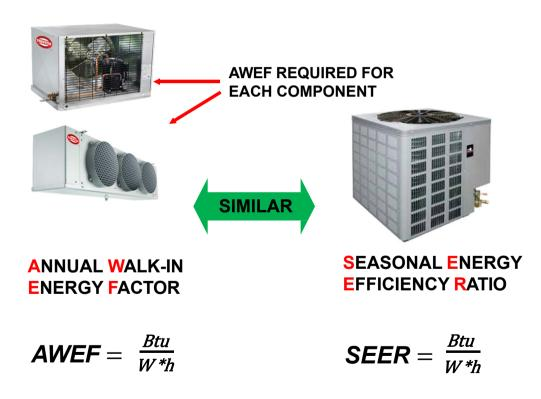
> The Annual Walk-In Energy Factor (AWEF) is a regulatory efficiency metric created by the Department of Energy (DOE) that measures electrical energy input versus the cooling capacity of the system.
